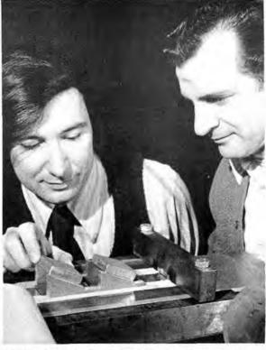
PRIOR TO IMPACT WELDING EXPERIMENT, Gene Neau (8342), left, and Gayle Cain (8415) place specimens above an exploding foil.
